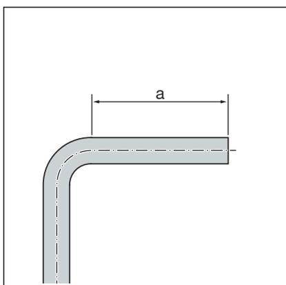
Pipes in the sizes d 15, 18, 22 and 28 can be bent cold with commercially available bending equipment (radius at least  $3.5 \times d$ ).
