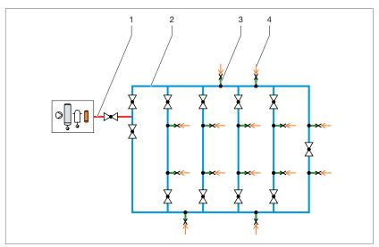
Fig. 128: Compressed air supply with ring system
