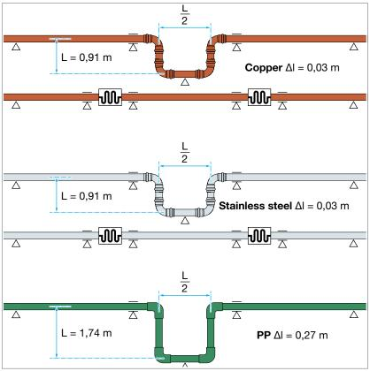
Fig. 76: Linear expansion in piping
