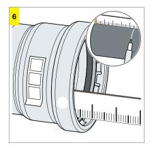
Measure the insertion depth and mark it on the pipe.
