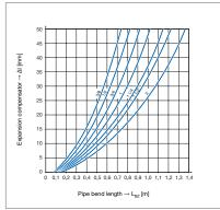
Fig. 52: U-shaped expansion bend for Megapress/Megapress S  $\frac{3}{-2}$  inches
