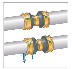
Fig. 191: SC-Contur using the Raxofix as an example
