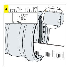
Mark the insertion depth on the pipe.
