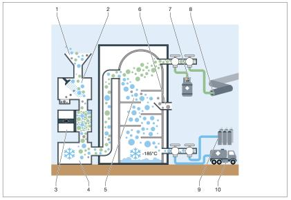
Fig. 138: Principle of an air separation unit
