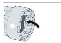
Fig. 23: Insertion of the sealing element into press connectors – up to 2 inches
