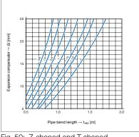
Fig. 50: Z-shaped and T-shaped expansion bends for Megapress/ Megapress S %–2 inches
