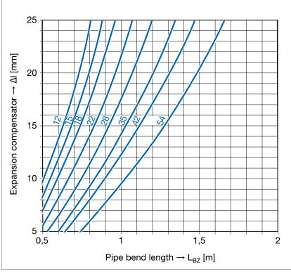
Fig. 79: Z-shaped or T-shaped expansion bend
