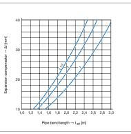
Fig. 51: Z-shaped and T-shaped expansion bends for Megapress S XL 2½–4 inches
