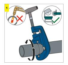
Cut the steel pipe properly and at a right angle using a pipe cutter, angle grinder or finetoothed hacksaw. Do not use a flame cutter.
