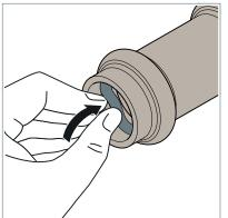
Fig. 13: Insertion of sealing element into press connectors – 12–54 mm
