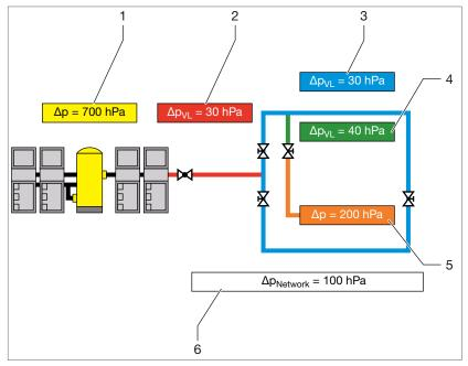
Fig. 130: Pressure losses from a compressed air system
