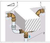
Fig. 157: Bypass around an obstacle
