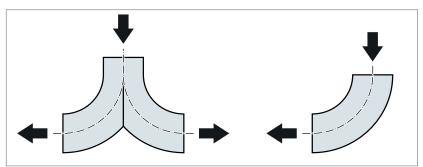
Fig. 132: Y-section and elbow
