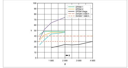
Fig. 10: Compression set for various EPDM types at the same temperature during the test procedure according to DIN EN 681-1
