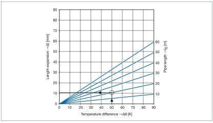
Fig. 35: Linear expansion of 1.4521/1.4520 stainless steel pipes
