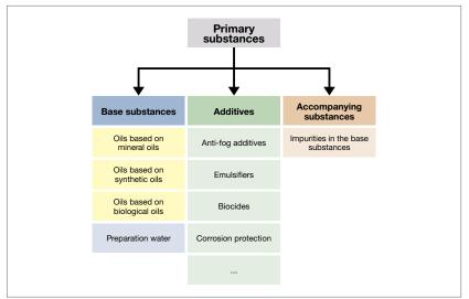
Fig. 165: Primary substances of the cooling lubricants (CL)
