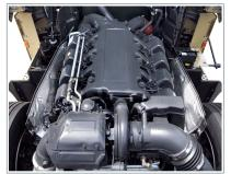
Fig. 169: Truck diesel engine
