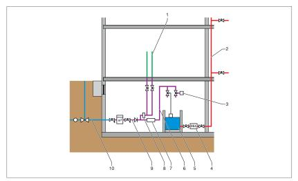
Fig. 108: Firefighting water transfer point with direct connection to the potable water installation
