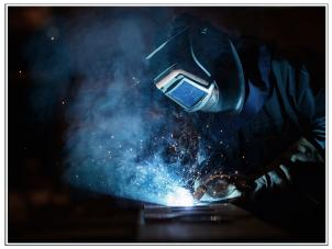
Fig. 135: Gas metal arc welding
