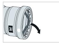
Fig. 25: Removal of the sealing element from press connectors – from 2½ inches
