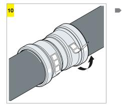
Remove the control label to mark the connection as "pressed".
