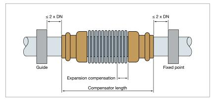
Fig. 55: Dimensions of axial compensators
