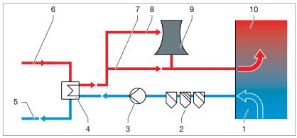
Fig. 93: Through-cooling
