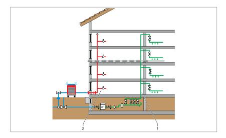
Fig. 110: Firefighting water system dry
