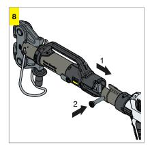
Place the Press Booster in the press machine and lock in place using the retaining bolt.
