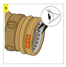
Ensure the sealing element and cutting ring are properly seated.
