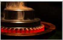
Fig. 136: Protective gas furnace for hardening gearwheels
