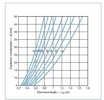
Fig. 40: Length determination for U-shaped expansion bend
