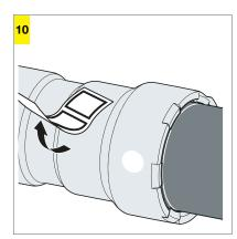
Remove the control label to mark the connection as "pressed".
