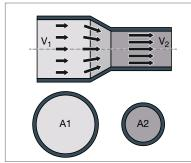
Fig. 126: Flow behaviour in case of changes to the cross section
