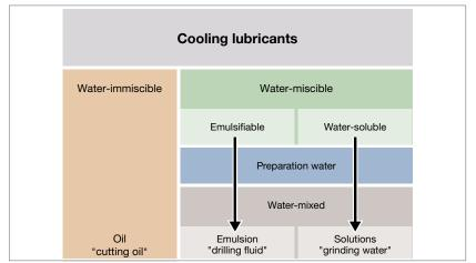
Fig. 166: Types of cooling lubricant (CL)
