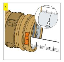
Mark the insertion depth on the pipe.
