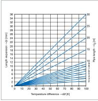
Determination of the expansion bend length for steel piping from % up to 4 inches
