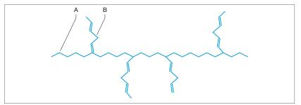
Fig. 3: Schematic representation of EPDM
