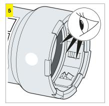
Ensure sealing element, separator ring and cutting ring are properly seated.
