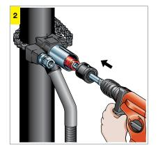
The hole is drilled by means of a commercially available drilling machine. The steel chips can be extracted by means of the vacuum cleaner nozzle. Afterwards, remove the drilling device again.
