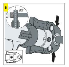
Place the Megapress press jaw (≤ DN25) around the press connector. Ensure it is properly seated. Carry out the pressing until the press jaw is completely closed.
