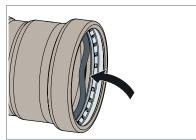
Fig. 16: Insertion of the sealing element into XL press connectors – 64.0–108.0 mm
