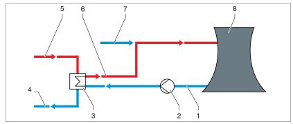
Fig. 94: Open cooling circuit with circulation cooling
