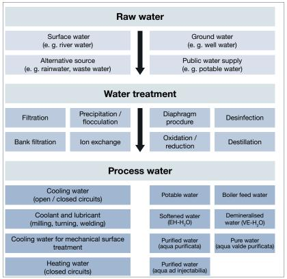
Fig. 88: Industrial process water supply
