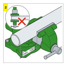
Caution when clamping! The pipe ends must be absolutely round.
