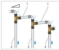
Fig. 154: Condensate discharge downwards
