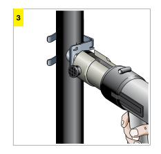
Press the press-in branch connector to the steel pipe by means of the press machine and the positioning aid. This is a fast and clean way of making the connection to the pipeline.
