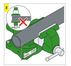
Proceed with caution when clamping the pipe – avoid deformation of the pipe end.
