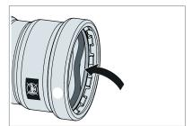
Fig. 26: Insertion of the sealing element into press connectors – from  $2\frac{1}{2}$  inches
