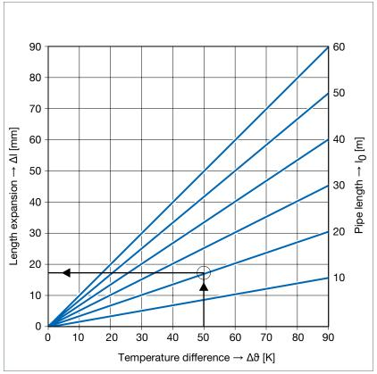
Fig. 78: Linear expansion of metal piping
