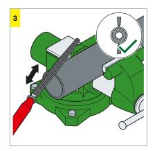
Properly deburr the inside and outside of the pipe.
