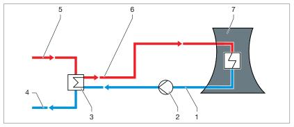
Fig. 95: Closed cooling circuit with circulation cooling
