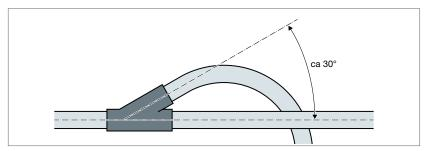
Fig. 133: Laying the connection line
