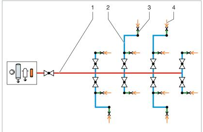
Fig. 129: Compressed air supply with single connection pipeline
