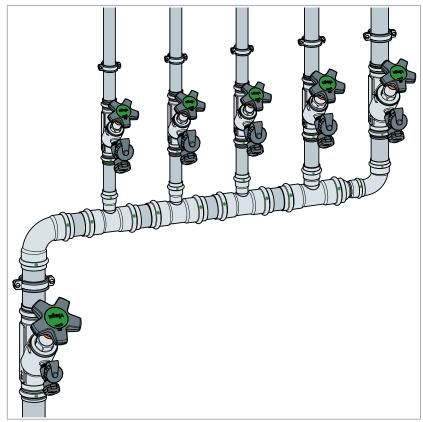
Fig. 80: Hygienically optimised manifold installation
