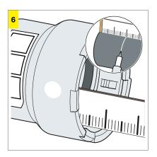
Measure the insertion depth and mark it on the pipe.
