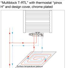
System illustration "Multiblock T-RTL" with surface heating
