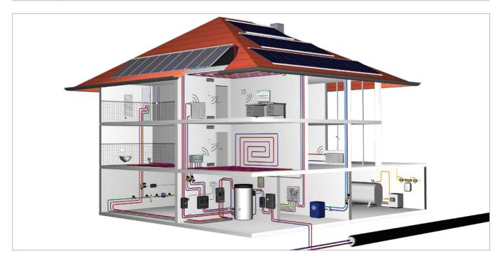
The variety and different models of Oventrop valves and controls allow the stockist, plumber and specifying engineer to fulfil all technical requirements concerning radiators, accessories and the complete heating system. Due to their presetting, they permit a hydronic adjustment of the flow rate and thus guarantee an economical heat output of the individual radiators.
