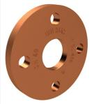
wetted metal parts made from dezincification-free and corrosion-resistant gunmetal, resistant against aggressive water, according to accepted materials list from German environmental agency, similar to DIN 2642, ÜA-Reg.-Nr. R-15.2.3-21-17048, WIEN-ZERT, pressure rating PN 16, max. operating temperature 200 °C
